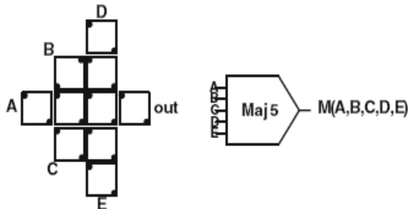
Figure 5. 5-input majority gate and its schematic
