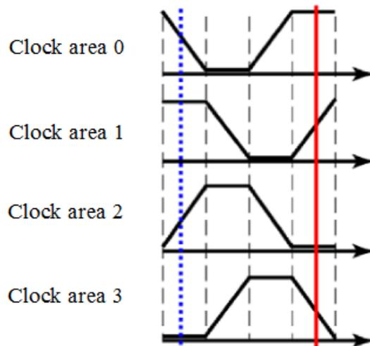
Figure 2. Four clock signals necessary for controlling QCA circuits
