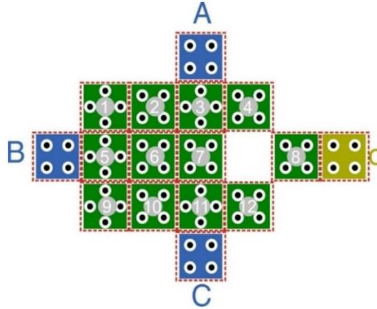
Figure 8. The proposed fault tolerant 3-input majority gate (numbered cells)
