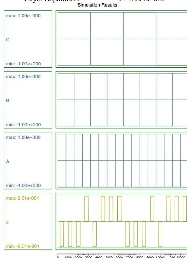
**Figure 7. The simulation result of the proposed fault tolerant 3-input majority gate**
