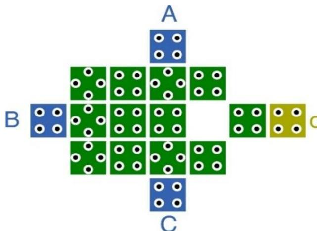
Figure 6. The proposed fault tolerant 3-input majority gate
