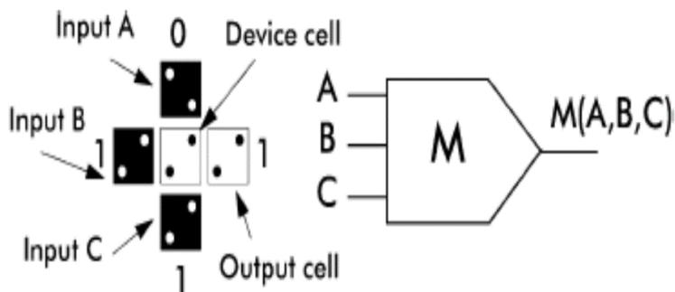
Figure 4. 3-input majority gate and its schematic
