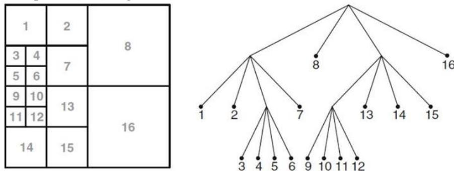
*Figure 1. Architecture of tree structured PUs in 3D-HEVC.*
