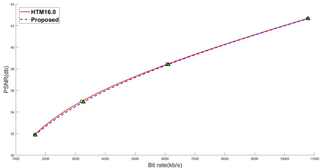
*Figure 11. Results of bit-rate and PSNR in Shark video (1920x1088) with different QPs*
