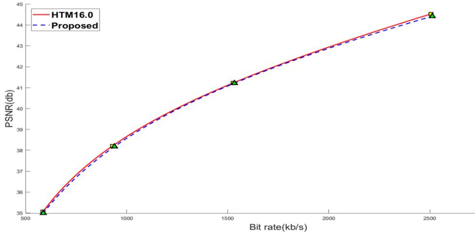
Figure 9. Results of bit-rate and PSNR in Kendo video (1024×768) with different QPs
