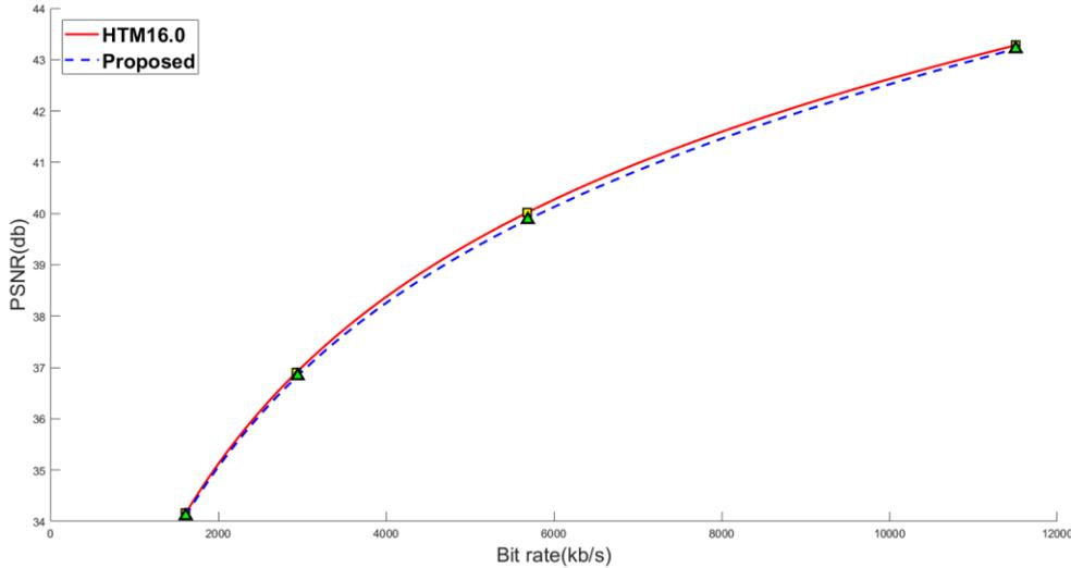
Figure 7. Results of bit-rate and PSNR in Poznan street video with different QPs
