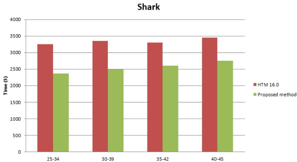
*Figure 10. Simulation results of Shark video (1920x1088) with different QPs*
