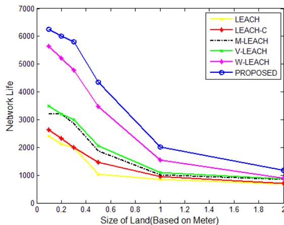
Figure 9: Network Life According Various Size of Land in Proposed Method and LEACH, LEACH-C[13], M-LEACH[16], V-LEACH[17], W-LEACH Protocol[18].
