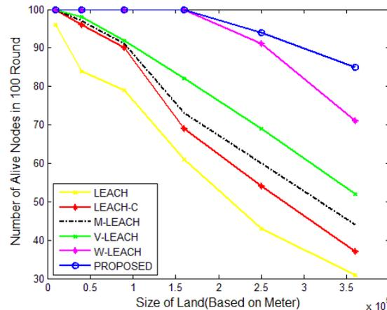
**Figure 10: Number of Alive Nodes According Various Size of Land in Proposed Method and LEACH, LEACH-C, M-LEACH, V-LEACH, W-LEACH Protocol**
