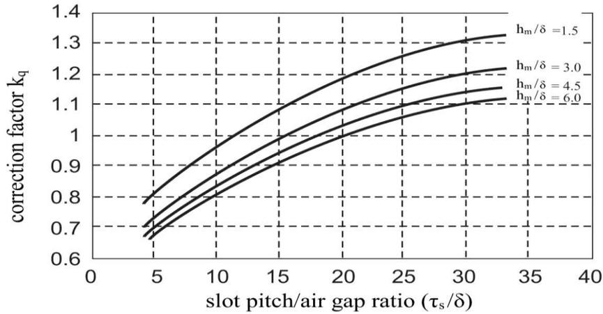
Fig. 2: Determination of  $k_q$
