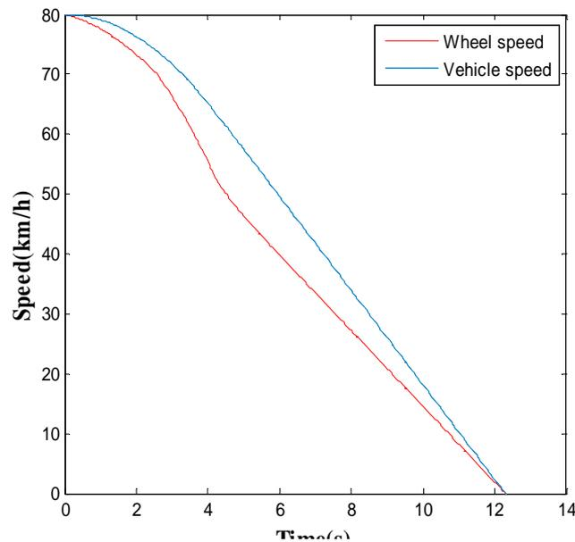
Figure 14. Wheel and vehicle speed for icy road
