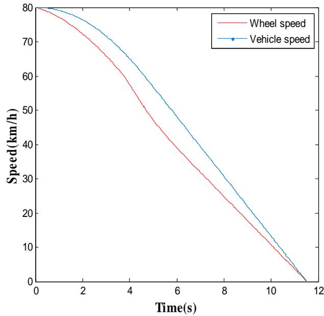
Figure 13. Wheel and vehicle speed for dry road
