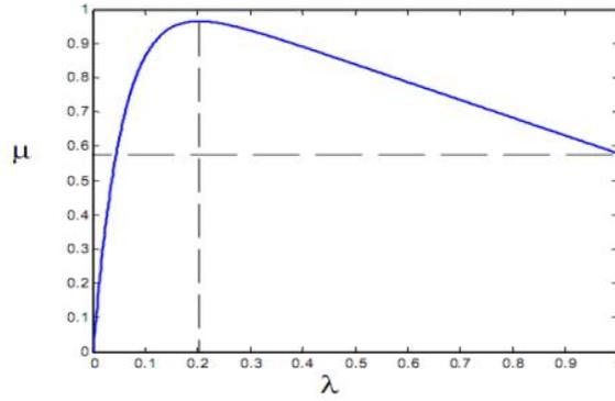
Figure 1. Dependence of friction coefficient on slip ratio
