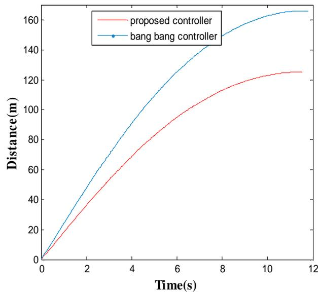
Figure 9. Stopping distance for dry road
