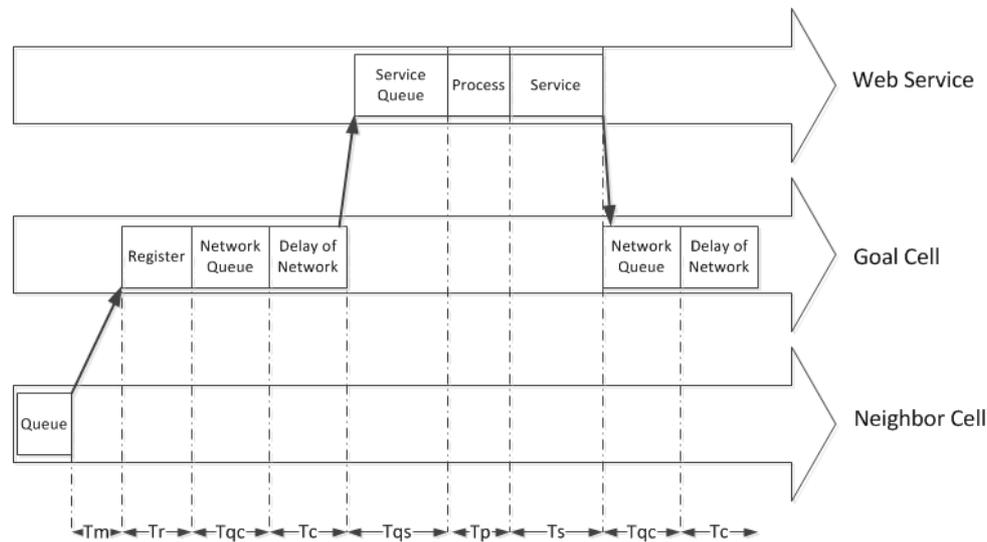
**Figure 2: Mobile agent request process in communication network**
