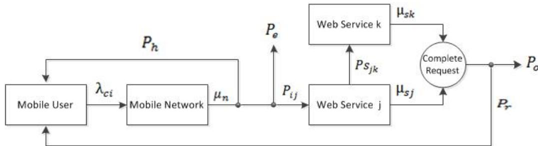
Figure 4: Mobile environments performance model
