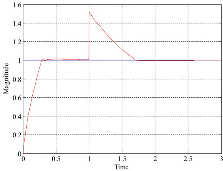
**Figure 11. Disturbance rejection**
