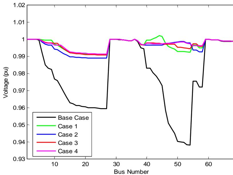
*Figure 15. Voltage profile for four DG installation cases and the base case for Winter-Night load level in 69-bus system*
