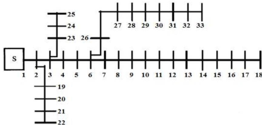
Figure 6. Single line diagram of a 33-bus radial distribution system
