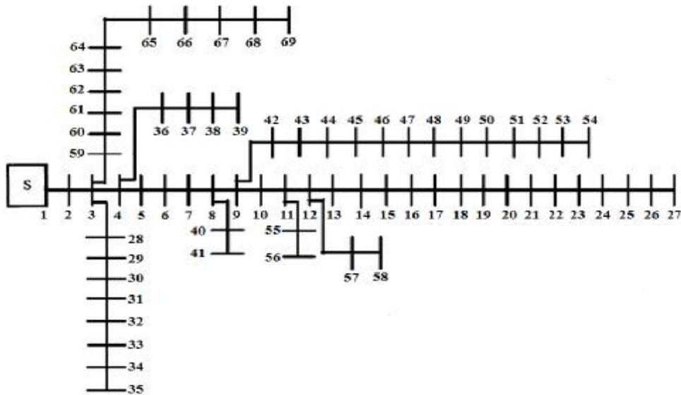
Figure 11. Single line diagram of a 69-bus radial distribution system
