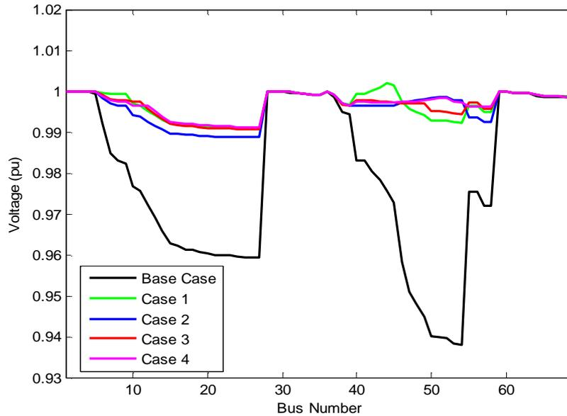
**Figure 12.** Voltage profile for four DG installation cases and the base case for Summer-Day load level in 69-bus system
