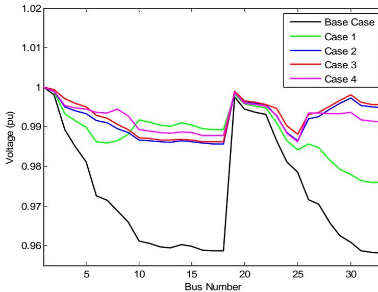
Figure 7. Voltage profile for four DG installation cases and the base case for Summer-Day load level in 33-bus system
