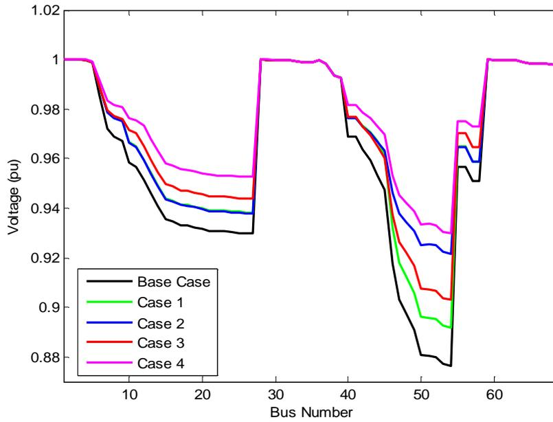
*Figure 14. Voltage profile for four DG installation cases and the base case for Winter-Day load level in 69-bus system*
