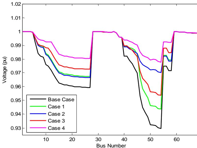
**Figure 13.** Voltage profile for four DG installation cases and the base case for Summer- Night load level in 69-bus system
