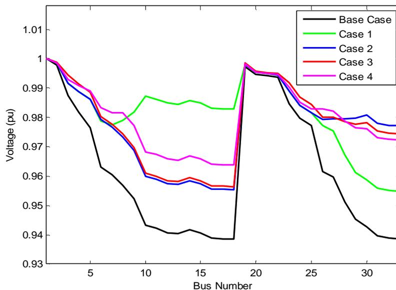
Figure 8. Voltage profile for four DG installation cases and the base case for Summer- Night load level in 33-bus system
