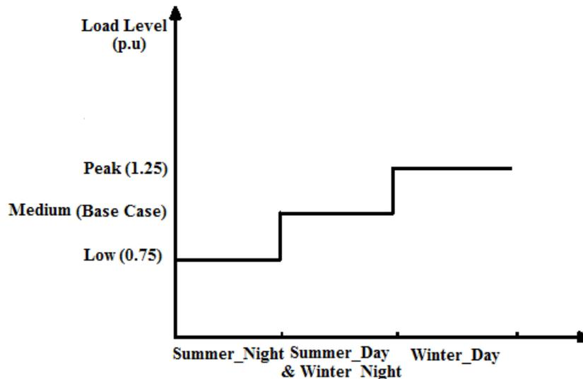
*Figure 1. Load level in different period of the year*
