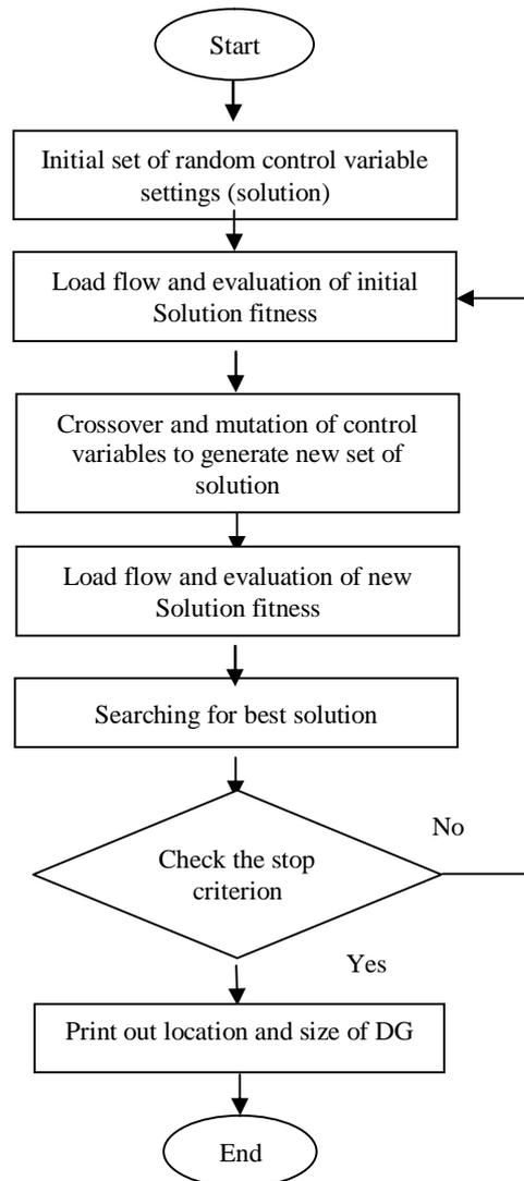
*Figure 5. Flowchart of Genetic Algorithm for placement problem*
