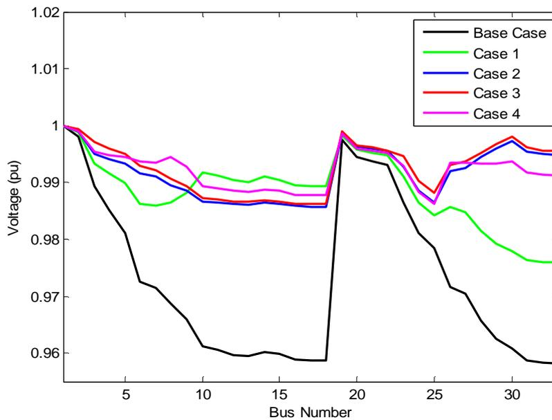
*Figure 10. Voltage profile for four DG installation cases and the base case for Winter-Night load level in 33-bus system*
