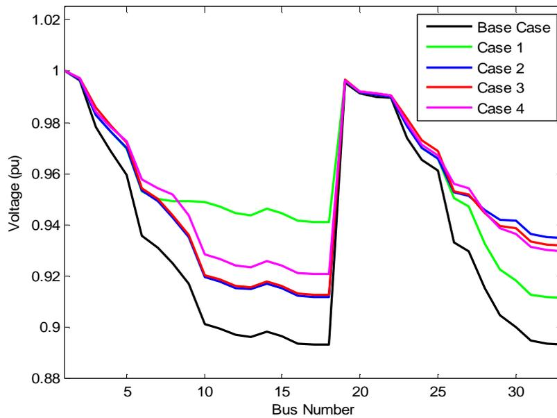
*Figure 9. Voltage profile for four DG installation cases and the base case for Winter-Day load level in 33-bus system*
