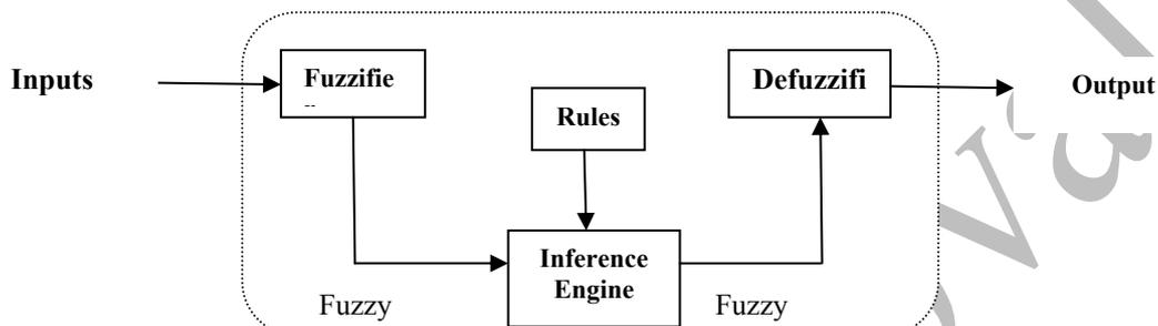
Figure 1. The architecture of fuzzy expert system
