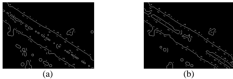
Figure 5. Results from applying the Canny edge detector. (a) From image Figure 4c (b) from image Figure 4d.
