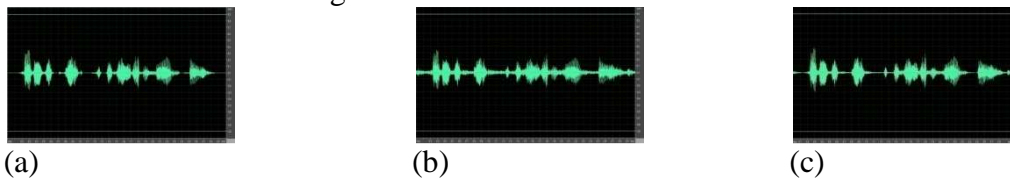
Fig 5. The time domain representation of (a) an arbitrary clean speech signal, (b) the speech signal which is corrupted by a 10 dB Babble noise process, (c) the noise reduced speech with SNR= 13.7 dB
