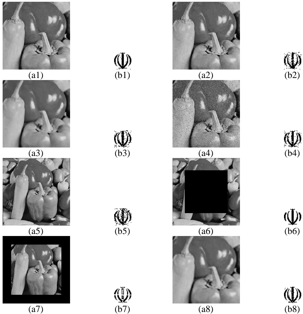
Figure 5. (a1), (a2), (a3), (a4), (a5), (a6), (a7) and (a8) watermarked image is degraded respectively through JPEG2000 compression, JPEG compression, median filtering, adding Salt&Pepper noise, rotating, center cropping, surrounding cropping and scaling. (b1), (b2), (b3), (b4), (b5), (b6), (b7) and (b8) The corresponding extracted watermarks.
