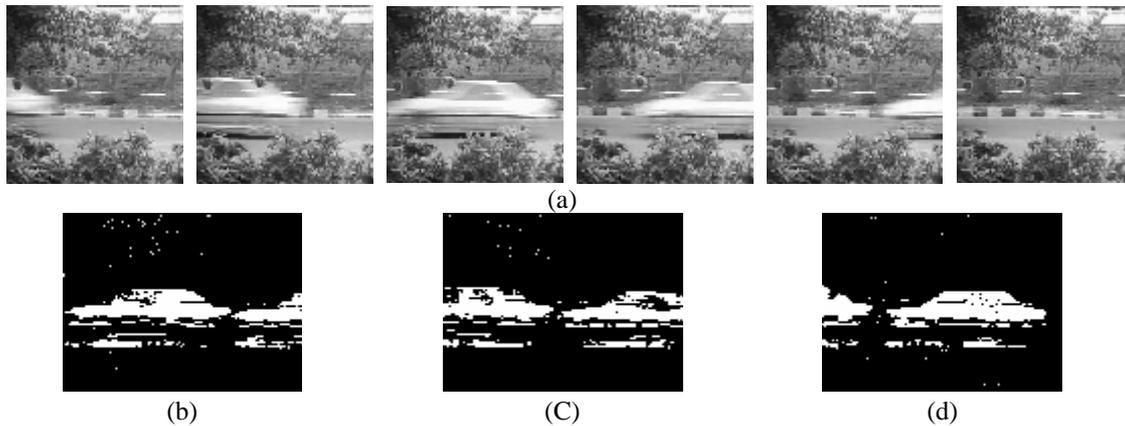
**Figure 3.** (a) Frames in which the car moves along the initial place completely (b) The difference of the first and the 4<sup>th</sup> frame (c) The difference of the second and the 5<sup>th</sup> frame (d) The difference of the third and the 6<sup>th</sup> frame.
