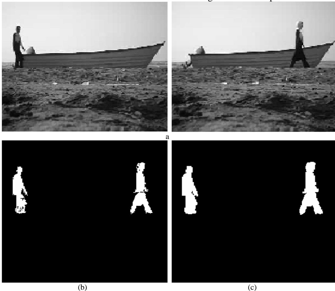
**Figure 1.** (a) Frames with similarity between colors of background and foreground in some regions, (b) The differenced frame (c) expanded detected regions.
