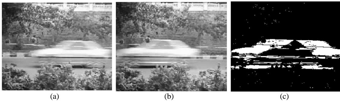
**Figure 2.** (a, b) Frames with overlap in the position of foreground objects (c) Differenced frame.
