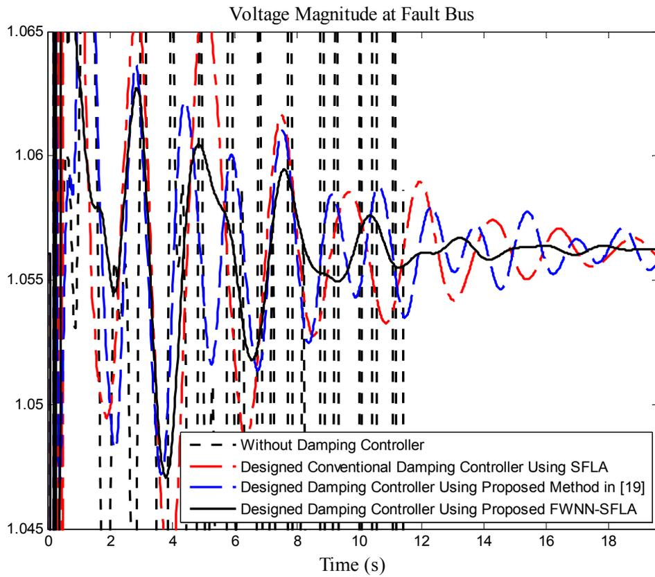
Figure 18. The response of the system to three-phase fault at bus 26.
