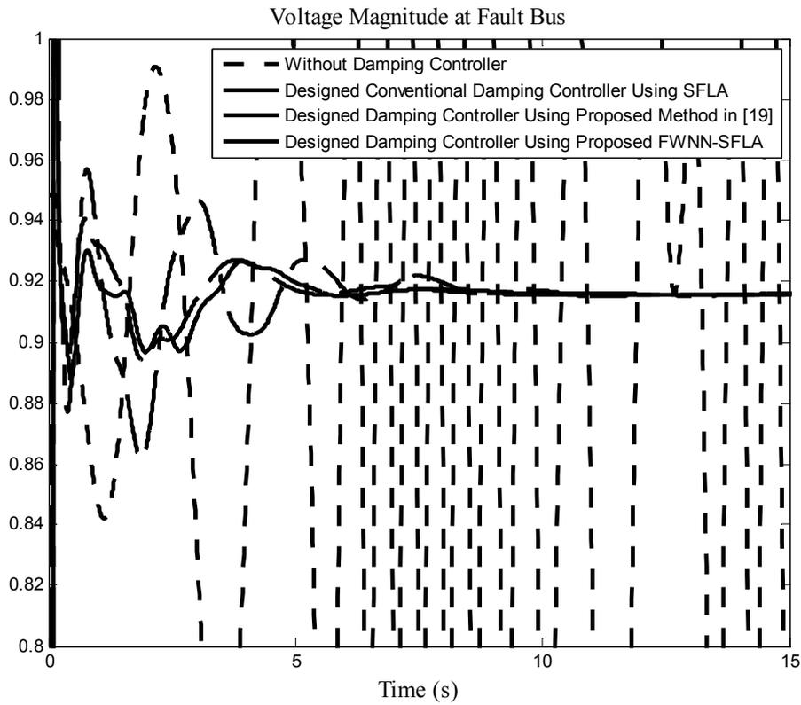
Figure 12. The response of the system to a three-phase fault at bus 3.
