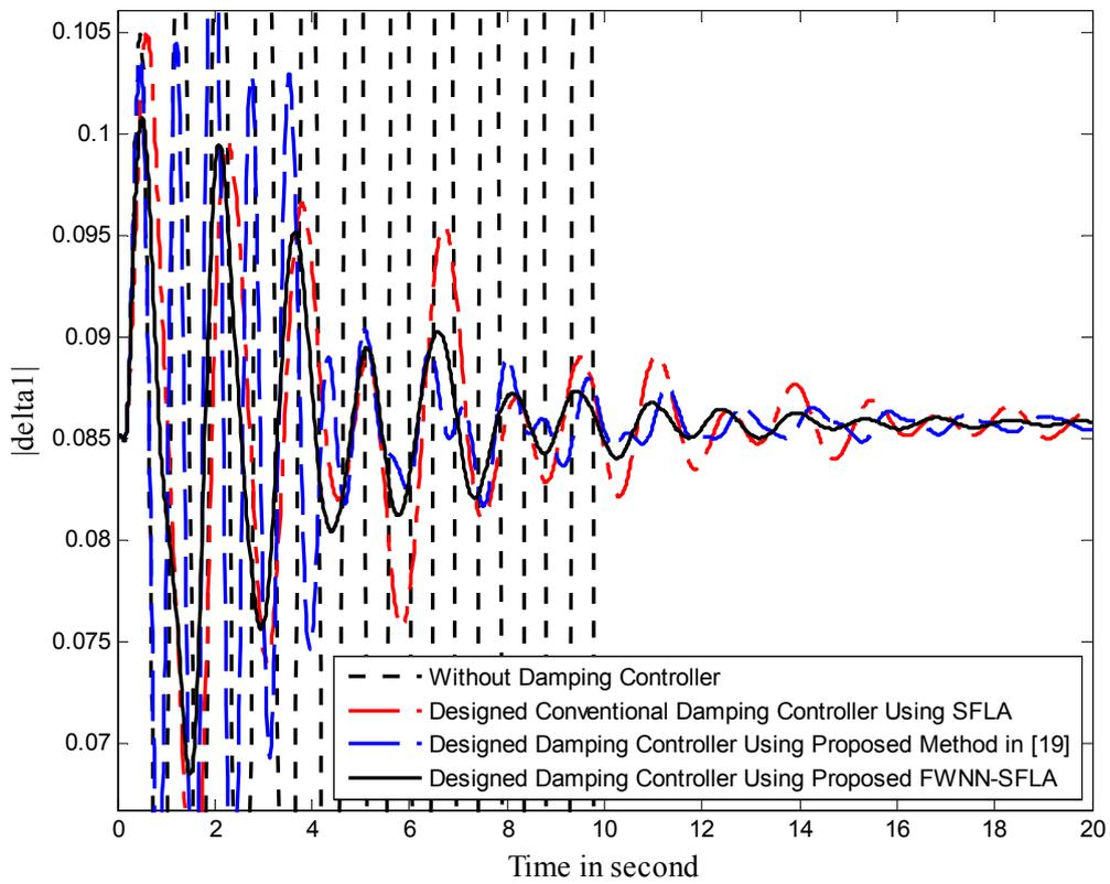
Figure 16. The response of generator 1 to a line-to-ground fault at bus 26.
