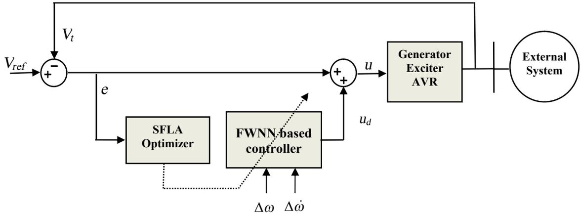
Figure 5. The proposed FWNN damping controller scheme.
