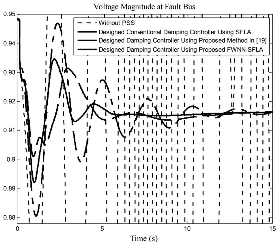
**Figure 9.** The voltage response of the system to a line-to-ground fault at bus 3.
