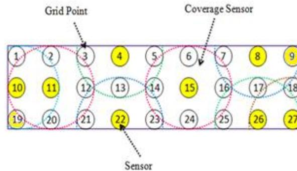
Figure 12. sensor area coverage with 9 × 3 grid points which is obtained using GLA
