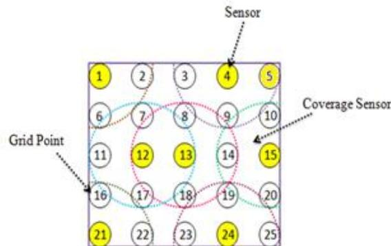
Figure 13. sensor area coverage with 5 × 5 grid points which is obtained using GLA
